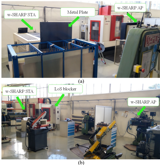
Fig. 12. Photos of the mechanical workshop used to test the PER and jitter. (a) Scenarios 1 and 2 (without and with the metal plate), (b) scenario 3.
