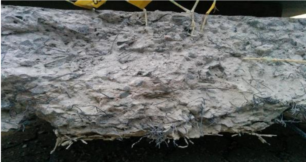
Figura 14. Steel fiber-reinforced concrete cross section
