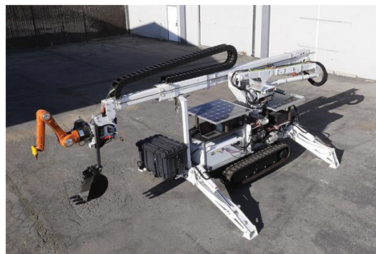
Figura 24. Digital Construction Platform ( money.cnn.com/2017/05/02/technology/3d-printed-building-mit/ )
