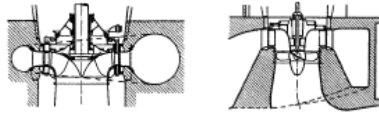
Figura 37. Francis (left) and Kaplan turbine (Minor, H.-E., 2008)
