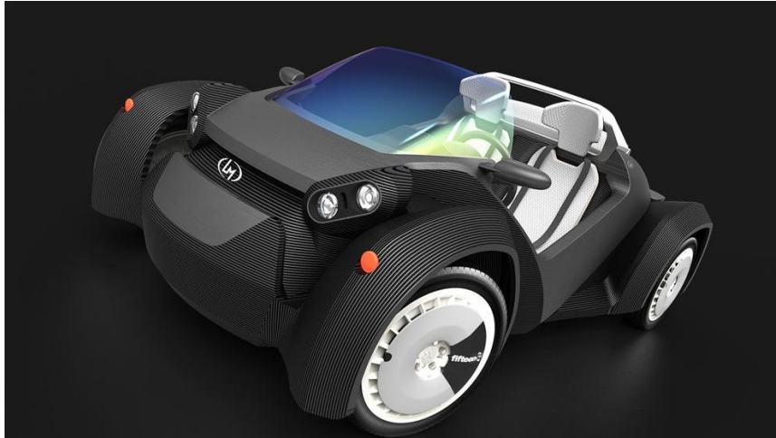
Figura 22. 3D printed car by Local Motors using carbon fibers (launchforth.io)
