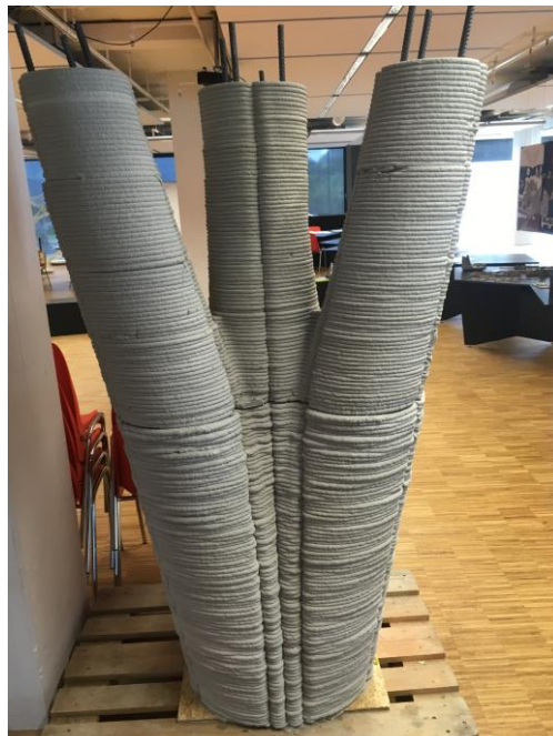
Figura 21. Column built through 3D printing with steel reinforcement
