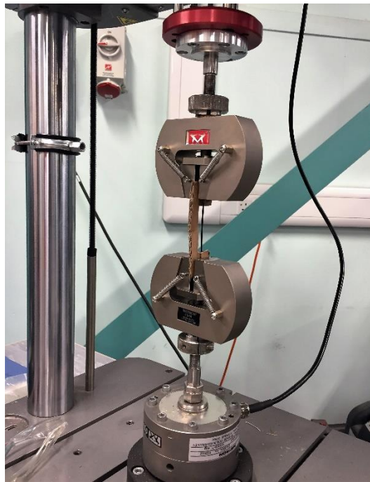
Figure 23: Filament sample mounted in Instron tensile testing machine
