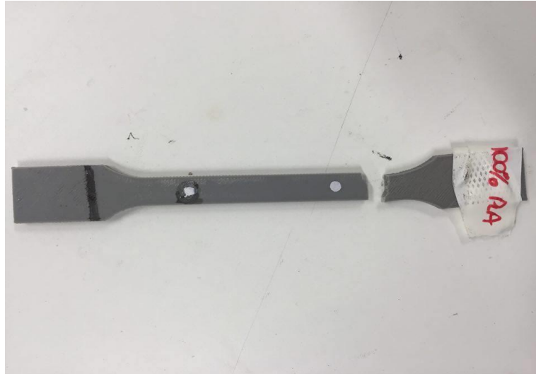
Figure 25: Example of a specimen that has broken outside of the gauge length
