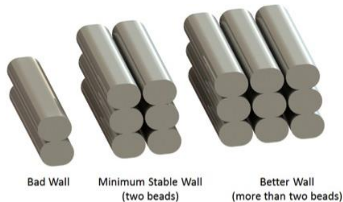
Figure 11: Schematic showing different wall thicknesses [21]
