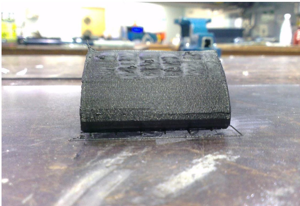
Figure 65: Example of poor print performance achieved using orientation 2
