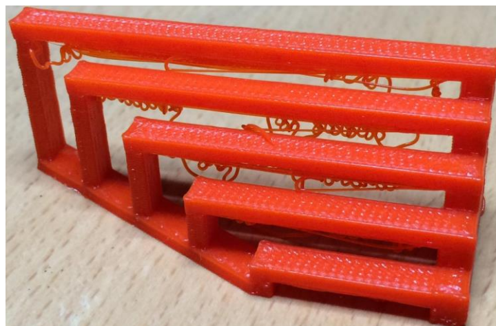
Figure 7: Example of printed component with bridging [22]
